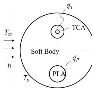
Fig. 2: Schematic of the thermal model.
