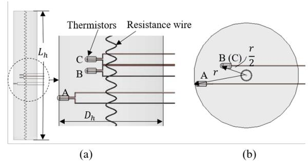
Fig. 5: Experimental setup to measure the convective heat transfer coefficient  $h$ . (a) The detailed front view. (b) The cross-section view.
