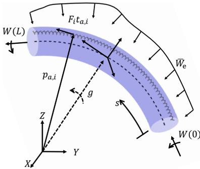
Fig. 3: Diagram for a Cosserat Rod.  $g$  represents the transformation from the fixed frame to the body frame. The internal wrench is  $\mathbf{W}$  and the distributed wrench is  $\bar{\mathbf{W}}_e$ . The force and the position in the TCA are represented by  $F_i \mathbf{t}_{a,i}$  and  $\mathbf{p}_{a,i}$ . The variable  $s$  is the spatial parameter varying from 0 at the base to  $L$  at the tip.
