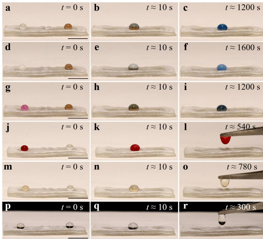
**Fig. 4** Biofluid droplet manipulation. (a–c), (d–f) and (g–i) On-demand, remote and lossless in-plane simultaneous mixing of BSA, milk and virus replicon particle-laden droplets, respectively, with Bradford reagent (right; reddish brown) to demonstrate protein detection. (j–l), (m–o) and (p–r) On-demand, remote and lossless in-plane simultaneous mixing of whole blood, PRP and fibrinogen droplets, respectively, with thrombin (right) to demonstrate clotting. Scale bar represents 10 mm.
